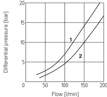
**7 DIAGRAMS OF JPR-3** based on mineral oil ISO VG 46 at 50°C
