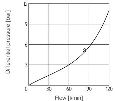
**6 DIAGRAMS OF JPR-2** based on mineral oil ISO VG 46 at 50°C
