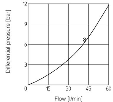
**5 DIAGRAMS OF KR-0** based on mineral oil ISO VG 46 at 50°C
