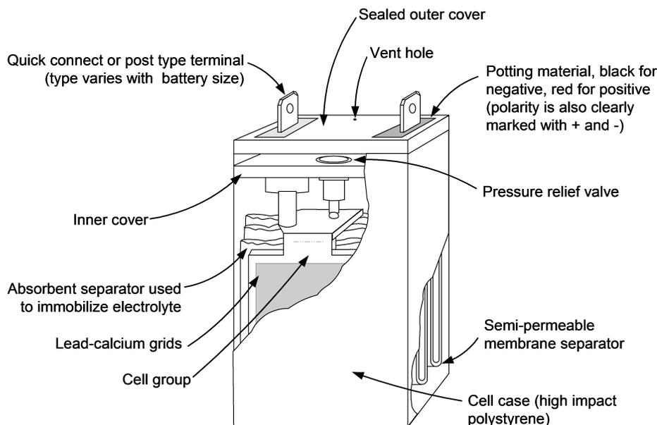
Figure 3: Battery construction reference
