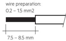
3.3 Wiring type and cross section for f version
