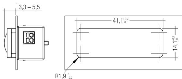
**3.5 Mounting in luminaire housing with Mounting Kit:**
