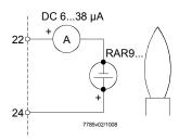
LGK16.../QRA53.../ QRA55... Use the KF8832 measuring device (not suited for continuous operation). There is no self-checking while measurements are made. The KF8832 is not required when using the QRA5x.D.../QRA5x.G...
