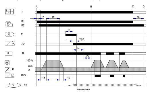
Interrupted pilot burners (burners with pilot burner), controlled and supervised by **LGK16.335** or **LGK16.635**, for example.
