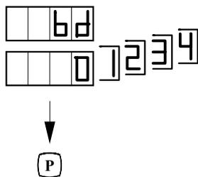
**3.24 Transmitting speed for serial interface (baud) (at 6490 / 3 / 4 and 6590 / 3 / 4)**
