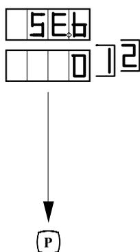
**3.20 Response to sensor failure PV (sensor break)**
