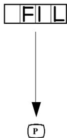
Software low-pass filter 1st order with adjustable time constant Tf to suppress interference signals and to smooth small process variable fluctuations.
