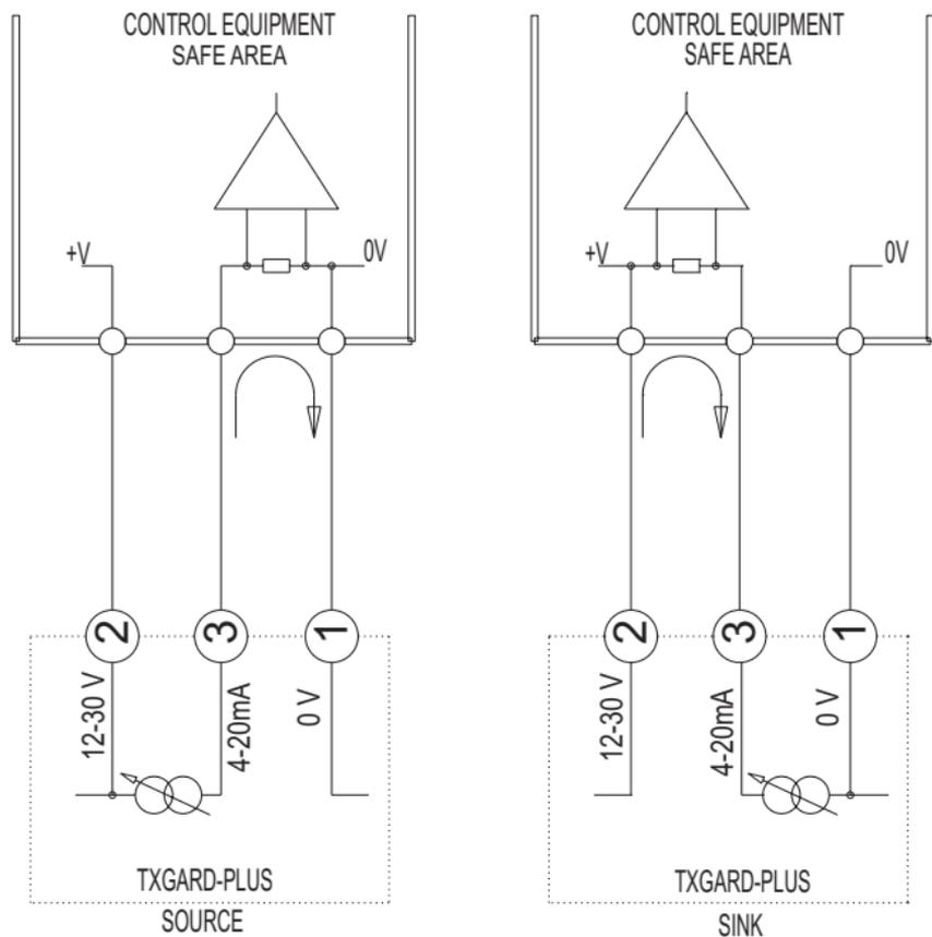
Diagram 3: Electrical connections to TXgard-Plus
