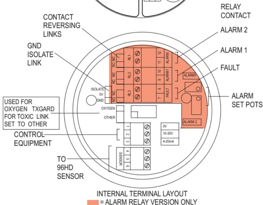
Diagram 2: Terminal and amplifier layouts
