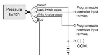
**Cautions:** 1. Use a stable DC power supply. If using switching power supply or other unit power supply, use with an FG terminal for the ground.
