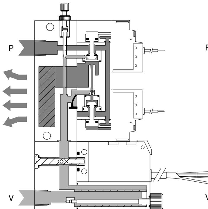
● When energizing a solenoid valve for controlling vacuum breaking air
