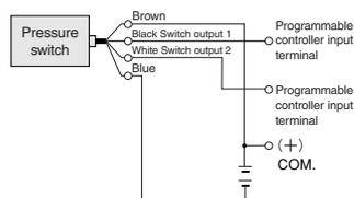
●GME-□EA Switch 1-output (variable hysteresis) + analog output type<sup>Note</sup>
