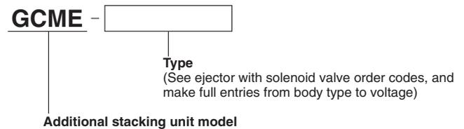
In addition to one manifold use ejector (GCME...), the additional stacking unit includes two stacking rods, one gasket, and one O-ring.
