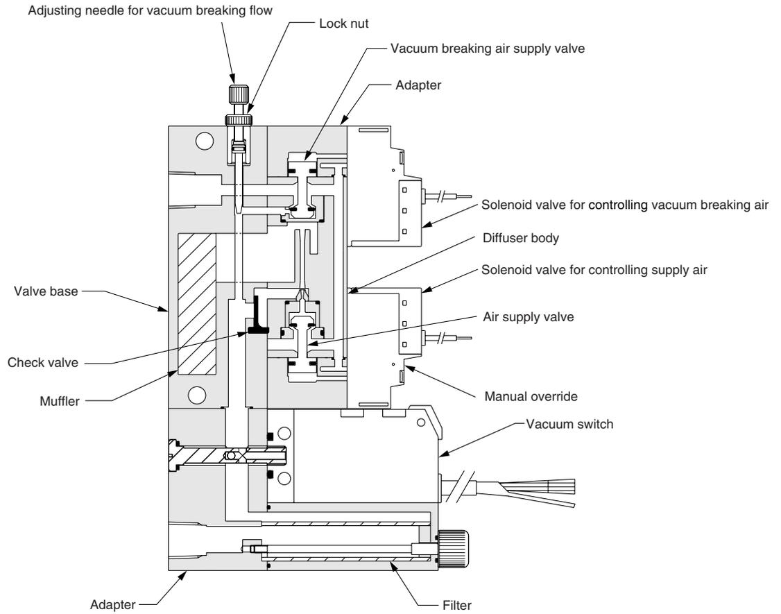
● When energizing a solenoid valve for controlling supply air (generating vacuum)
