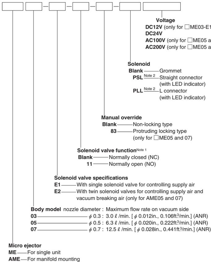
Notes: 1. Only for solenoid valve for controlling supply air. The solenoid valve for controlling vacuum breaking air is normally closed (NC) only.
