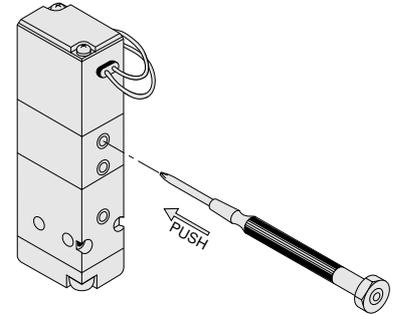
**Caution:** Always release the lock on the locking protruding type manual override before commencing normal operation.
