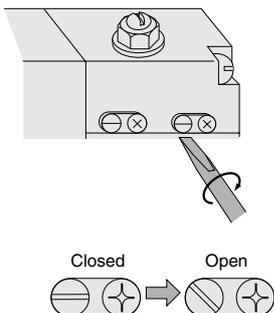
**Caution:** Always release the lock on the manual override before commencing normal operation.
