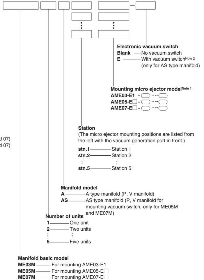
Notes: 1. For mountings of micro ejector options, see the micro ejector order codes. Also, if not mounting a micro ejector, and placing a block-off plate on the station instead, enter **-BP**.
