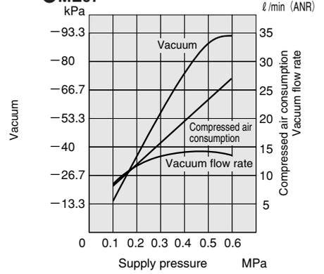
Remark: Graphs are for each single ejector unit. If the unit with solenoid valve requires the same vacuum level, set the supply pressure 0.03~0.05MPa [4.4~7.3psi.] higher than the single ejector unit's case.
