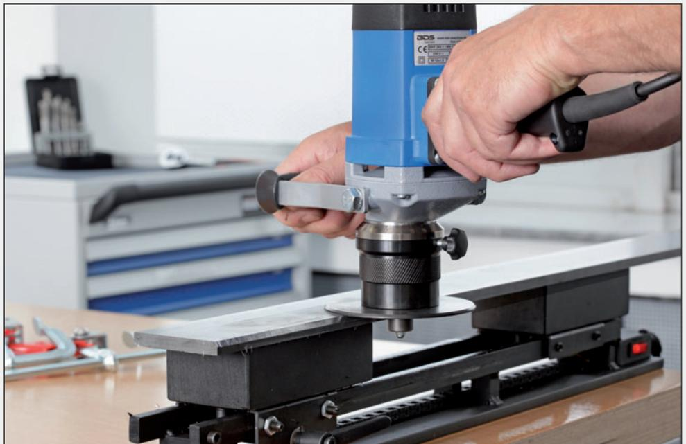
Edge processing with the EKF - the workpiece is securely fixed with the MagnetCLAMP magnetic clamping device. See page 79.
