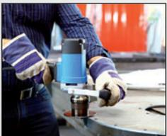
Three milling cutters with a chamfering angle of 45°, optionally 30° or a radius of 2.5 mm are available.
