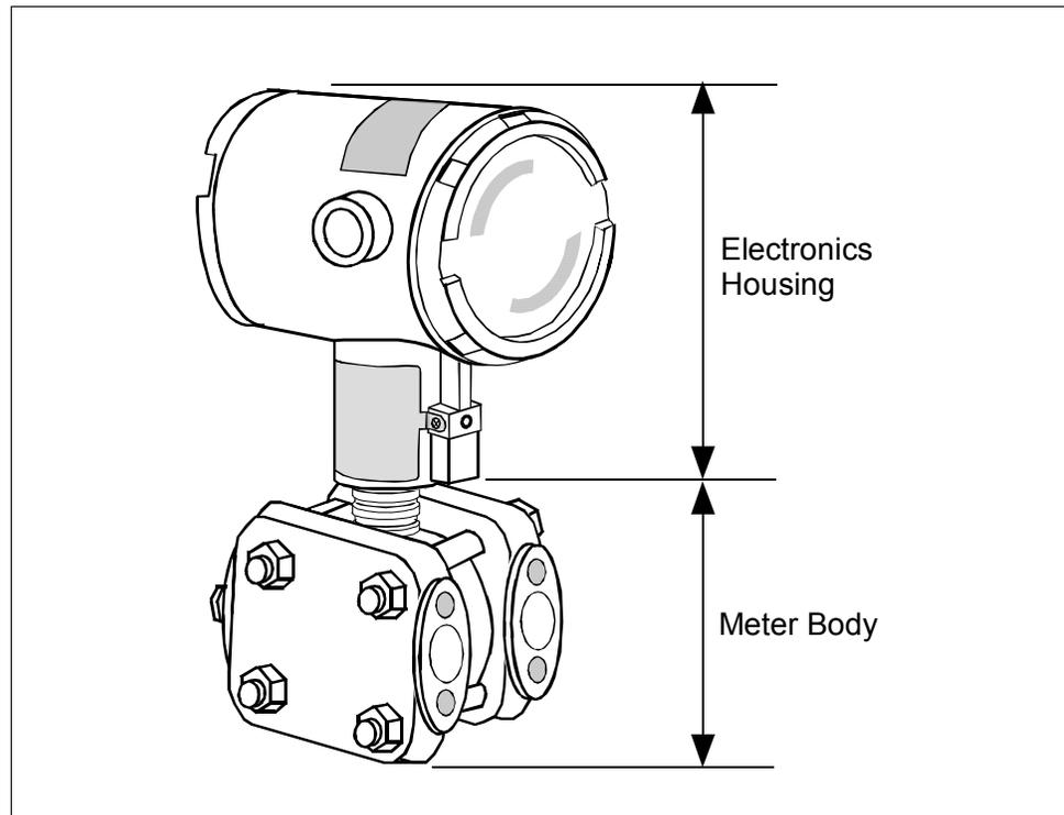
The ST 3000 can transmit its output in either an analog 4 to 20 milliamper format or a digital DE protocol format for direct digital communications with our TPS system, Allen-Bradley PLCs and other control systems.
