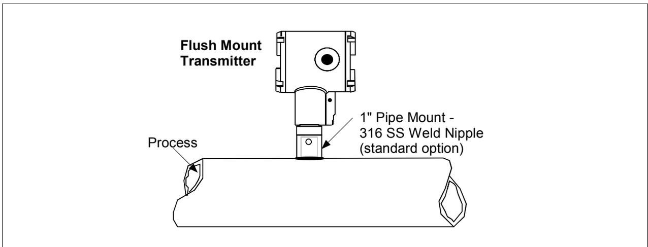
Figure 46 Typical Arrangement for Liquid Level Measurement with Flush Mount Transmitter
