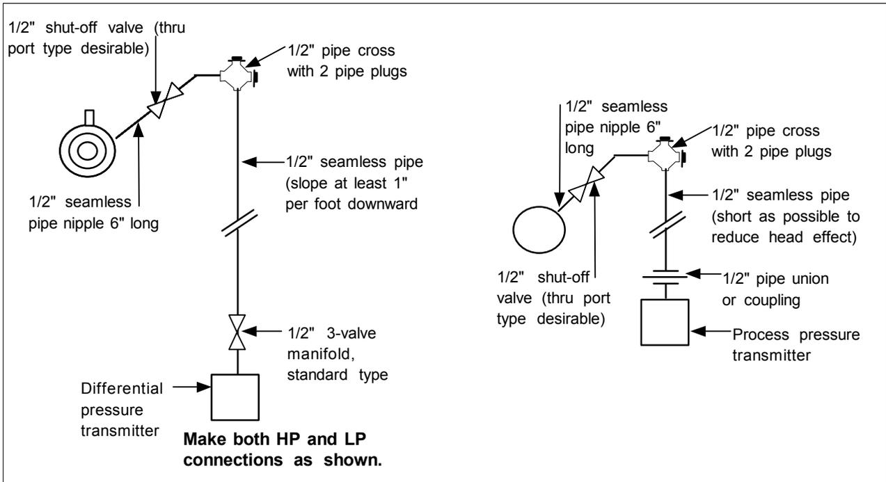
The installation should be checked every 6 to 12 months to verify that the sealing liquid is at its required specific gravity.
