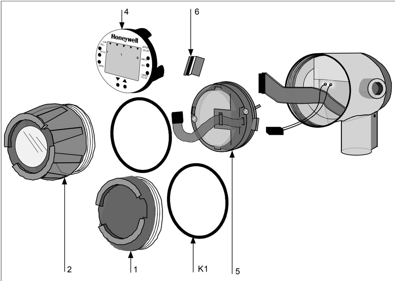
Figure 56 Series 100/900 Electronics Housing - Terminal Block End
