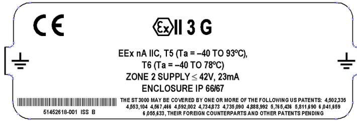
Nameplate 50003885-001, 4-20 mA / DE, multiple certification nameplate. The following is a representation of this nameplate:
