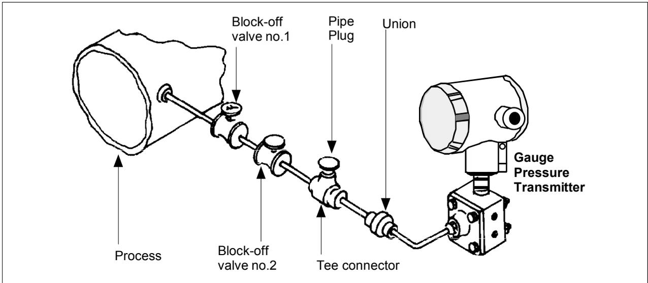
Figure 44 Typical Piping Arrangement for Liquid Level Measurement with GP Type Transmitter
