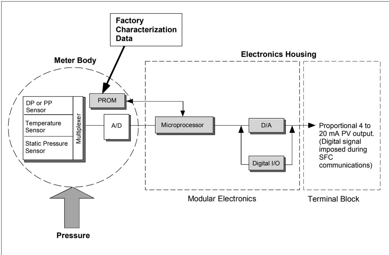
When the transmitter is in its DE mode, the process variable is available for monitoring and control purposes; and the meter body temperature is also available as a secondary variable for monitoring purposes only. See Figure 3.
