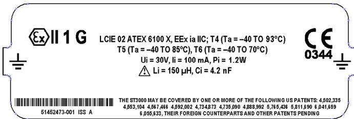
Nameplate 51452474-001, d, 4-20 mA / DE, is mounted on the enclosure. The following is a representation of this nameplate:
