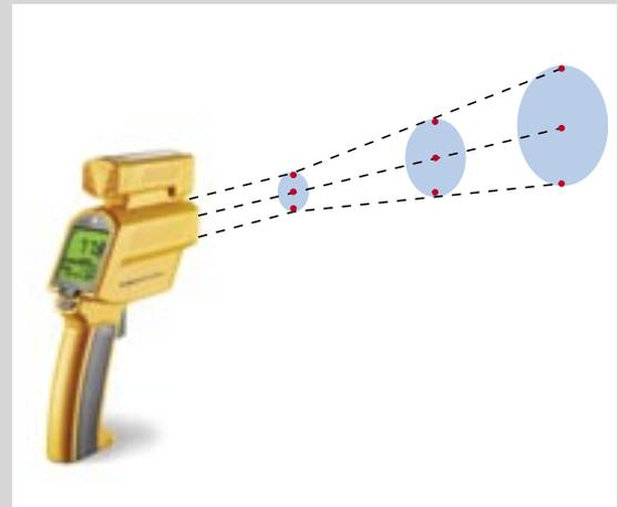
Accurate measurements depend in part on accurately sighting a target. Fluke 570 series thermometers are the only thermometers with a sighting system designed to precisely track the infrared path as seen by the sensors. This enables the advanced coaxial three-dot laser sighting to accurately show both the center and the edges of the spot being measured, regardless of the thermometer's distance from the target.
