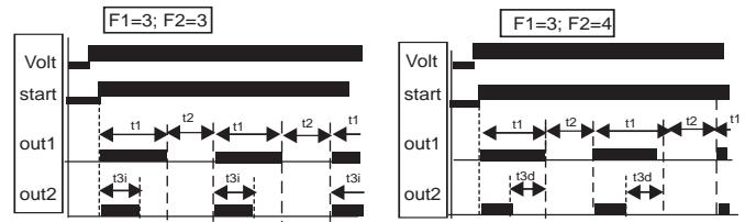
t1 and t2 works on the output OUT1 (T2 is available with functions with two times F1=3, 4, 5)
