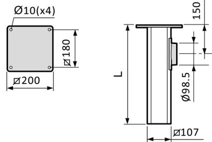
Ceiling bracket, for fitting through beams. The attachment plate is adjustable for the entire length of the aluminium profile. If required, the aluminium profile can be cut during fitting.
