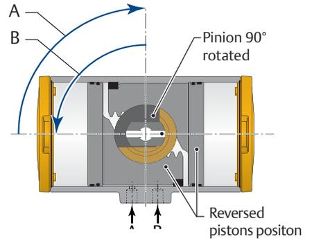
A = Rotation when central air chamber is pressurized.
