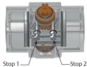
4. Turn the “closed” stop clockwise to reduce or counterclockwise to increase the travel. Consult Section 5.1.3 (angular displacement of the pinion), to define how far the limit stop must be turned in or out.
