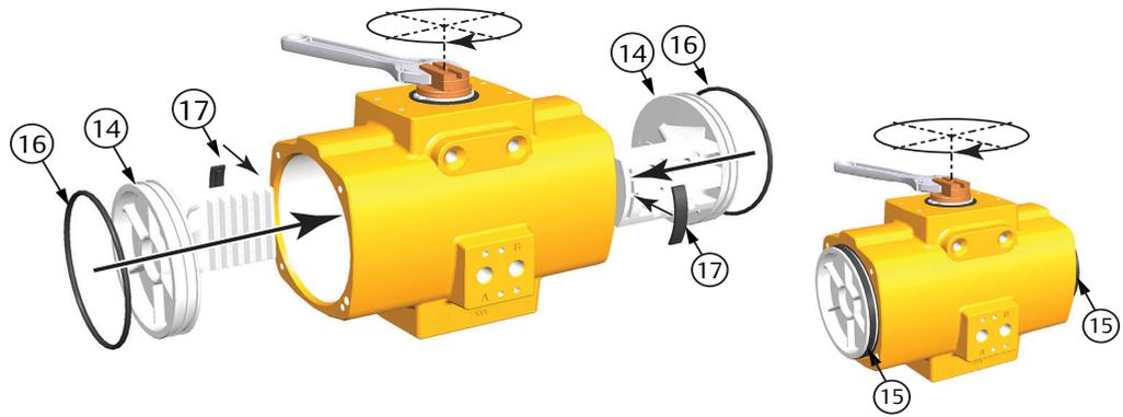
3. Align the pinion (see Figure 28) so that the teeth on the pinion will pick up the pistons rack teeth when turning the pinion. The position of the pinion top slot and the cam on the pinion top:
