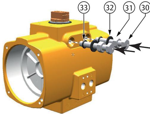
2. Move the pistons inward until the slot in the top of the pinion is perpendicular to centerline of the housing.
