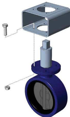
5. Install the actuator to the bracket. Tighten all bolts and apply the correct torque (refer to Table 8).
