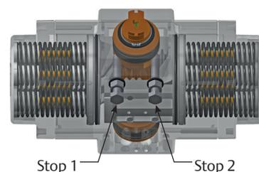
3. Turn the “closed” stop clockwise to reduce or counterclockwise to increase the travel. Consult Section 5.1.3 (angular displacement of the pinion), to define how far the limit stop must be turned in or out.
