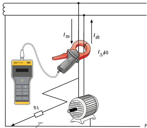
Abb. 3.2: Part of the current flows through an insulation fault  $R_f$ . The sum of the two currents is no longer zero. As soon as the residual current reaches or exceeds the response value there is an alarm message on the EDS195P.
