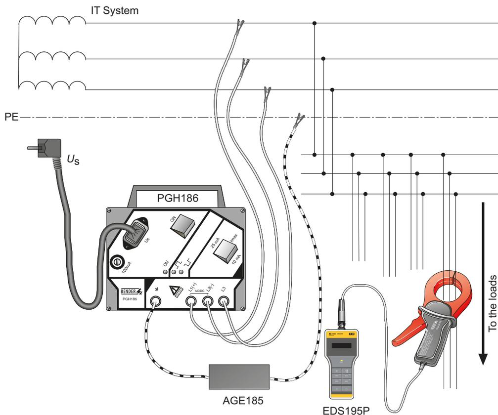
Abb. 6.3: Connection diagram EDS309... with AGE185
