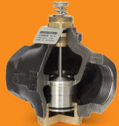
2TBB Series = 2-way valves, bronze body, with threaded connections up to 2", brass plug, stainless steel stem. Temperature applications -10°C to 130°C. Rangeability 50:1. To be motorised by MVE and MVH actuators (no adapter needed).
