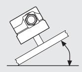
When installed in other position the pressure switch switches at pressure deviating from the set reference value by max.  $\pm 0.2$  in. W.C. (0.5 mbar).
