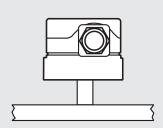
When installed horizontally, the pressure switch switches at a pressure higher by approximately 0.2 in. W.C. (0.5 mbar).
