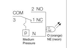
**GML** (Operating state shown) **As pressure falls**, 2 NO opens, 1 NC closes, Neon light ON (fault), switch trips and locks out.
