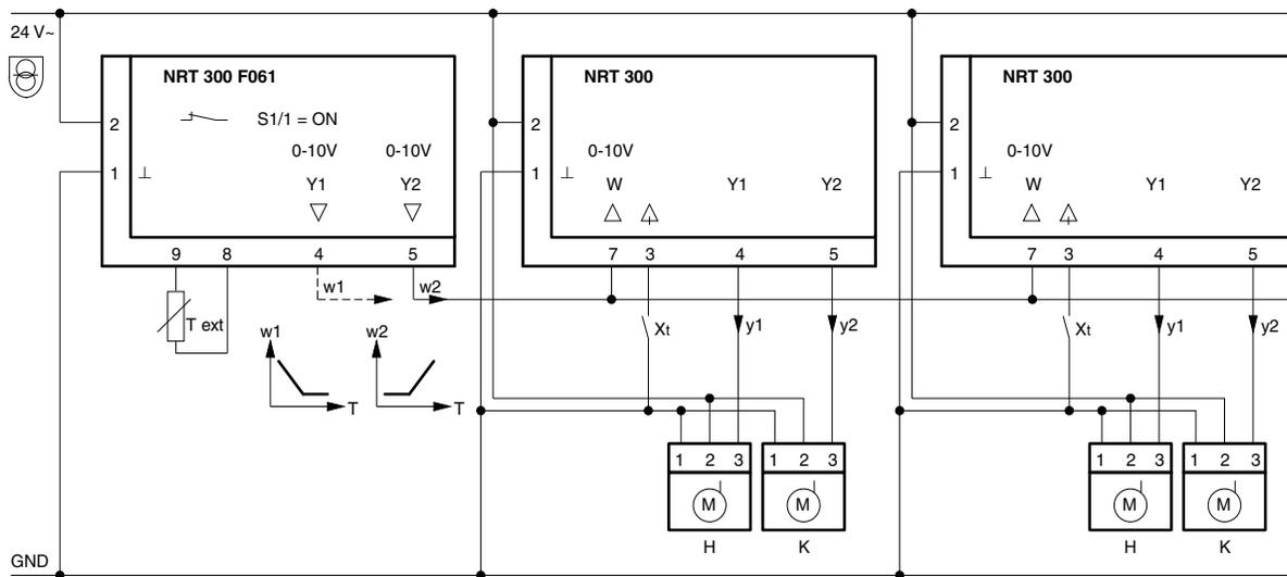
Outputs  $w_1$  ( $y_1$ ) and  $w_2$  ( $y_2$ ) (total load > 5 k $\Omega$ ) of the master controller to shift max. 10  $\times$  NRT 300
