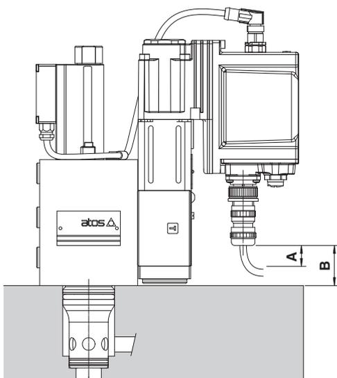
**A** = 15 mm space to remove the 7 or 12 pin main connectors
