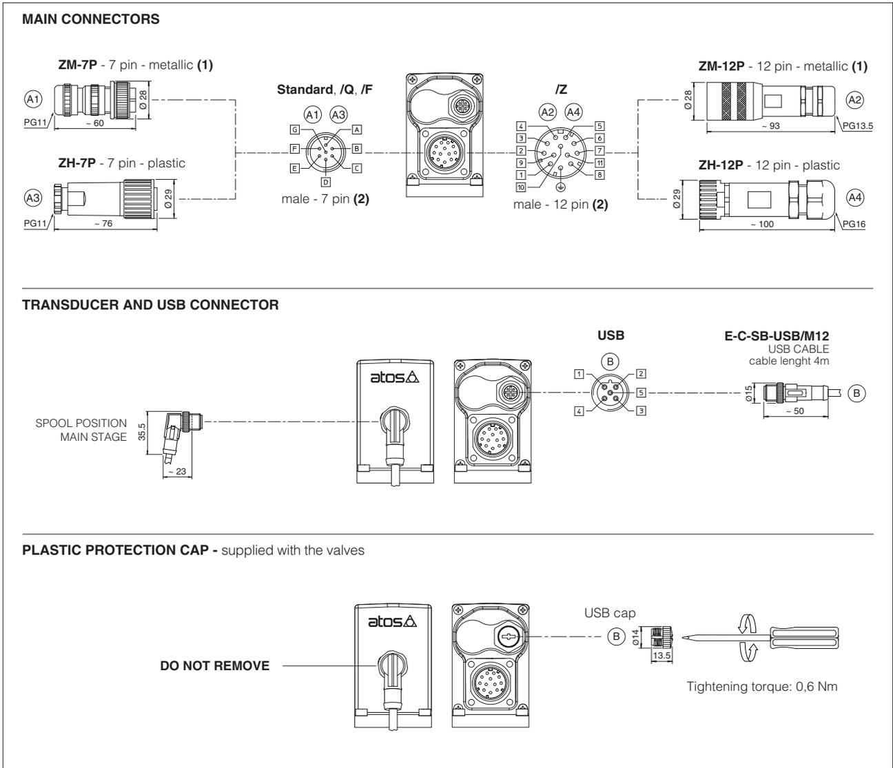
**(1)** Use of metallic connectors is strongly recommended in order to fulfill EMC requirements
