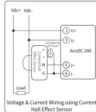
**NOTE:** Hall effect sensor can also be powered using the  $\pm 15V$  power supply in the X5 module.
