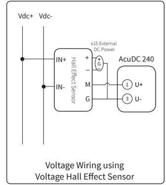
**NOTE:** Hall effect sensor can also be powered using the  $\pm 15V$  power supply from the X5 module.
