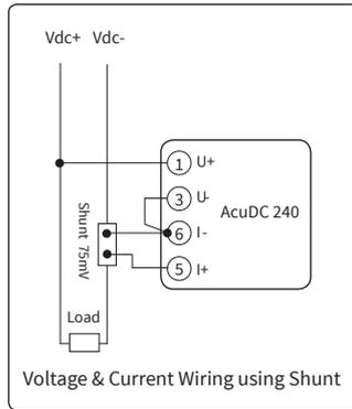
**NOTE:** A physical jumper from terminal 3 to 6 must be connected.
