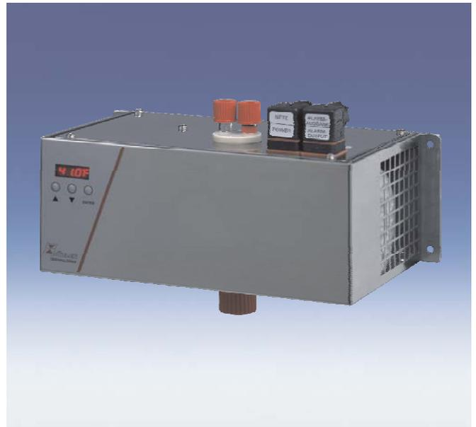
Accurate measurement of gases requires gas samples with stable dew points even under harsh ambient conditions. The PKE Models feature a semiconductor Peltier cooling system with an aluminum cooling block. Fitted into the block is a removable high efficient heat exchanger made of stainless steel, DURAN-glass or PVDF.
