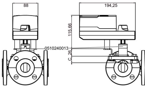
**MH32F and MH42F with actuator ASM 124**
