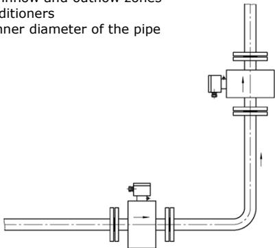
Fig. 2 Installation in horizontal and vertical pipeline
