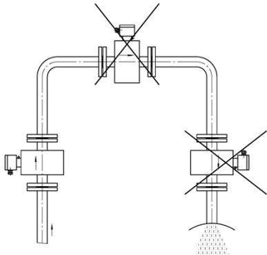
Fig. 3 Installation in risers and down pipes
