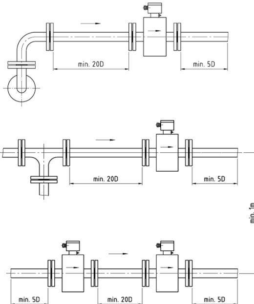
Fig. 5 Installation between tees, valves and pumps
