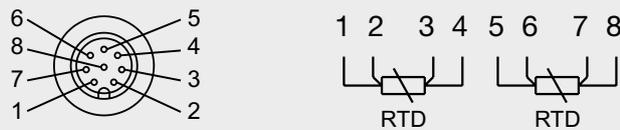
1x RTD with M12 plug for IO-Link operation
