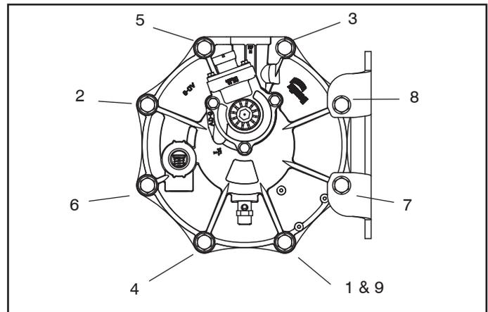
Figure 4 End Cover Bolt Torque Pattern
