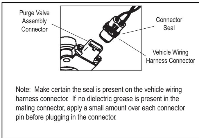
Figure 5 **Wiring Harness Connectors**
