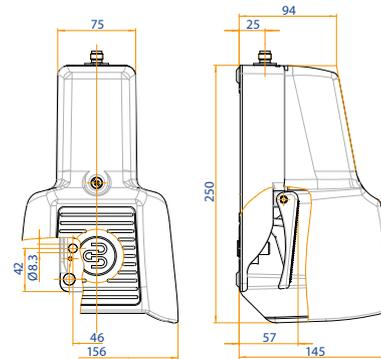
**21) Foot switch with safety lock + manual release F1 | Page 26**
