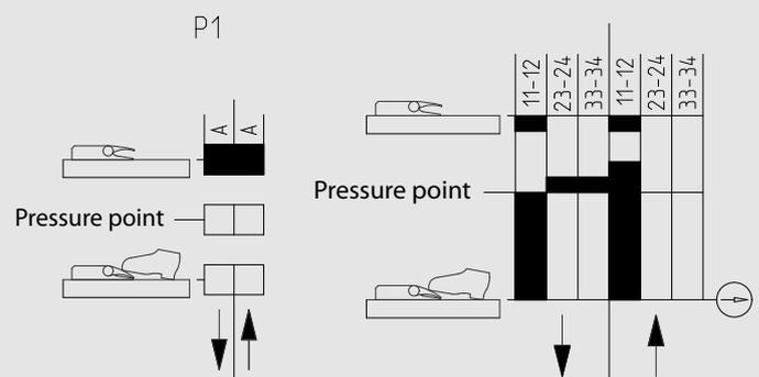
The indicated travels and forces refer to the switch-in contact of the foot switch with latching function.
