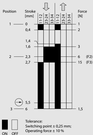
Switching diagram with PNP output
