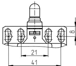
Mounting screw M5 according to DIN 912 or
