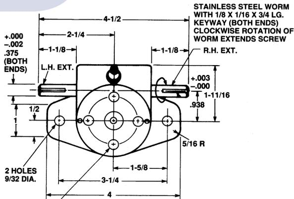
4 HOLES 9/32 DIA. EQUALLY SPACED ON 1-1/2 B.C.
