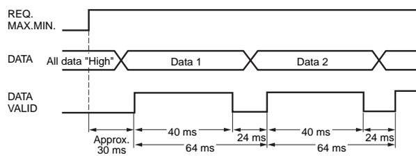
Measurement data is output every 64 ms while the REQUEST signal remains ON.
