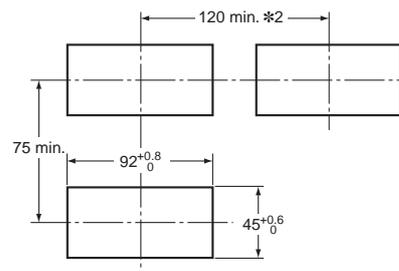
\*2. Leave a distance of at least 140 mm when using the Watertight Cover Y92A-49N.
