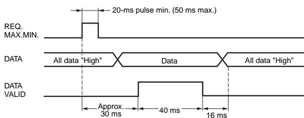
The data is set in approximately 30 ms from the rising edge of the REQUEST signal and the DATA VALID signal is output. When reading the data from a Programmable Controller, start reading the data when the DATA VALID signal turns ON. The DATA VALID signal will turn OFF 40 ms later, and the data will turn OFF 16 ms after that.
