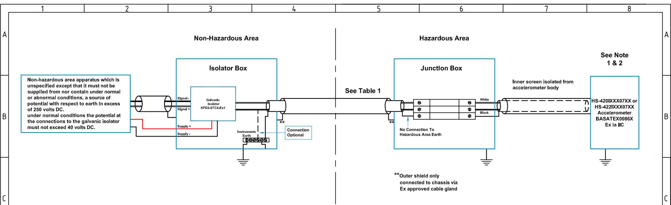
Non-hazardous area apparatus which is unspecified except that it must not be supplied from nor contain under normal or abnormal conditions, a source of potential with respect to earth in excess of 250 volts DC. under normal conditions the potential at the connections to the galvanic isolator must not exceed 40 volts DC.
