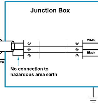
\*\*Outer shield only connected to chassis via Ex approved cable gland
