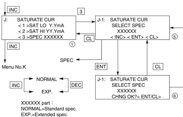
Saturation current value (Lower limit value=SAT LO, Upper limit value=SATO HI) and specification (SPEC NORMAL= Existing specification, SPEC EXP. = Extended specification) are settable.
