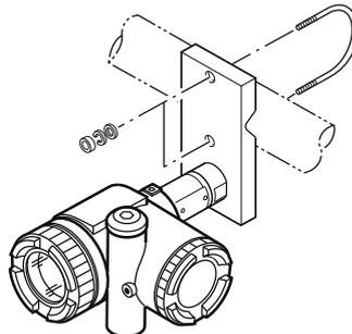
(1) Fasten the transmitter to a vertical or horizontal pipe using the supplied U-bolt (Tightening torque approximately 15 Nm (1.5 kgfm) <11ft-lb>).
