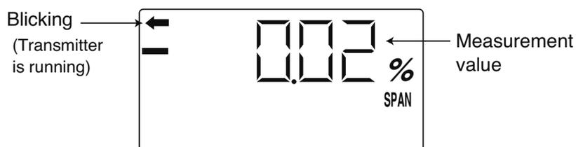
\* For status indication in the normal mode, refer to the previous section "Mode indicating function of digital indicator."
