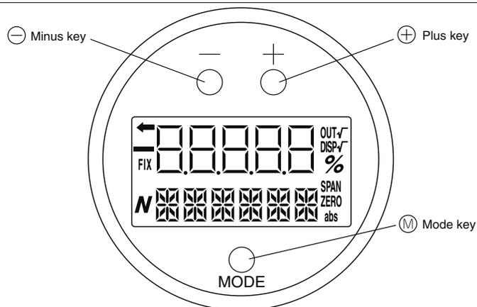
Normal mode (normal mode for indicating a measured value)
