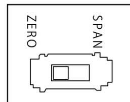
For zero suppression or elevation ranges, apply the specified pressure before adjust the 4/20 mA output signal using the external adjustment screw.
