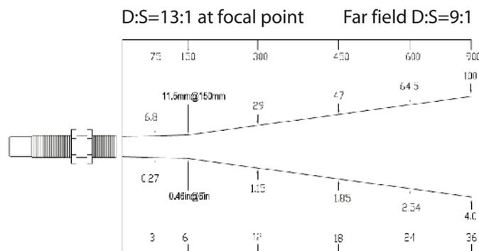
D:S is the optical resolution expressed as a ratio of the distance to the target spot divided by the diameter of the spot.
