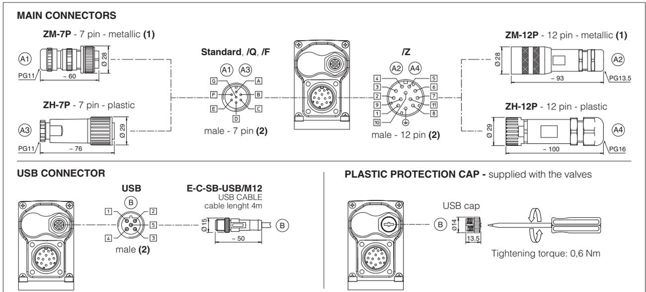
(1) Use of metallic connectors is strongly recommended in order to fulfill EMC requirements
