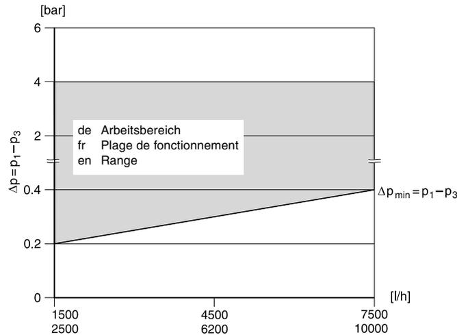
The required minimum differential pressure (min.  $\Delta p$ ) over the valve can be found in the diagram. The system can be set to this value precisely using the two pressure measurement nipples.
