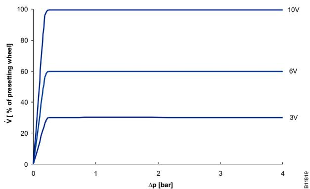
Example function: DN 40 VCL040F200 with preset max. volume flow 7500 l/h
