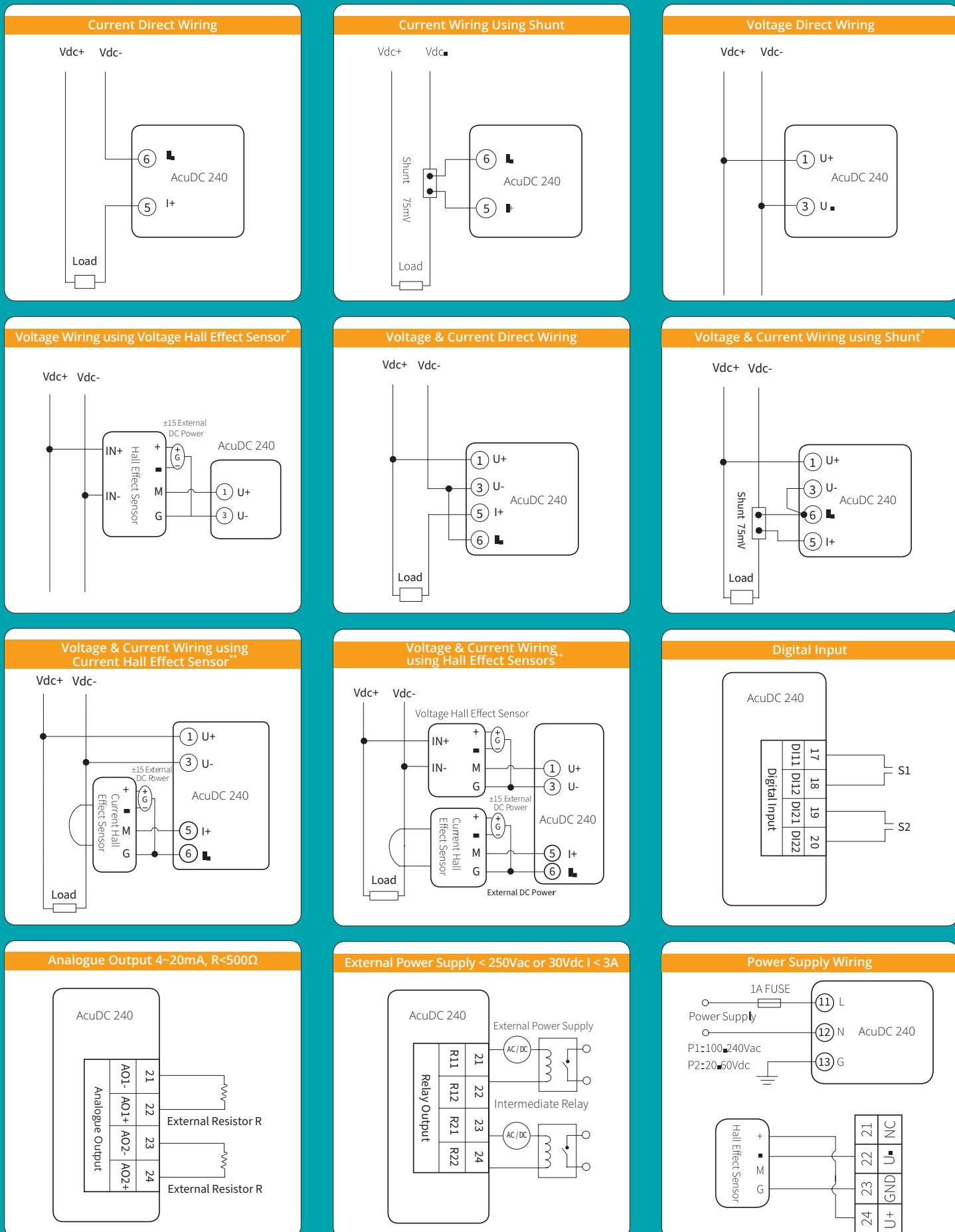
\*A physical jumper from terminal 3 to 6 must be connected.
