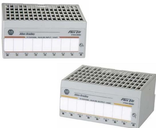
FLEX I/O™ HART modules provide your process automation system with full analog capability and the benefit of HART® (Highway Addressable Remote Transducer) protocol in an I/O module that can be used remotely. The modules offer 8 channels of analog input or output data with accompanying HART digital information.
