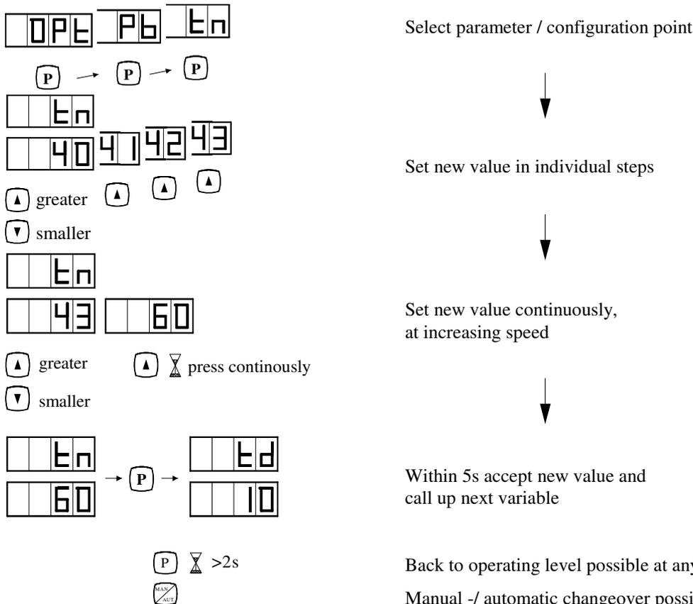
**3. Parameterization -/ configuration level**
