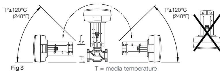
When media  $T^\circ$  exceeds  $120^\circ$  mount the actuator between  $45^\circ$  and the horizontal position (see drawing)
