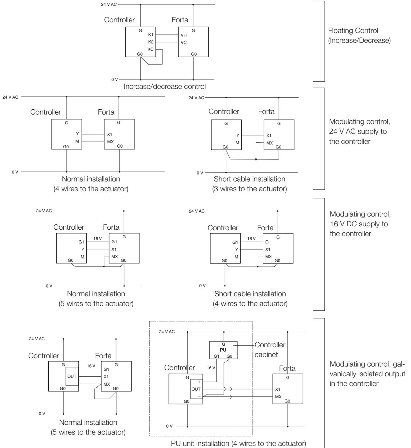
Fig 5 2...10V Feedback (Y) referenced to G0
