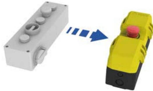
The EL AC series control stations by Pizzato Elettrica can be fitted with a new-concept flip-open protection cover, which allows the actuating devices to be safeguarded from knocks or dirt (often found in lift installation areas), while leaving the mushroom emergency button always accessible, even with the protection in the closed position. The cover is hinged on the right or the left side, and is provided with a snap system which prevents it from being closed unintentionally due to vibration.
