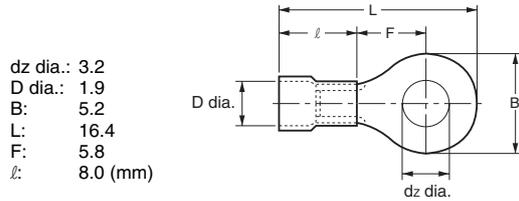
**Wiring (Ground Terminal Models)**
