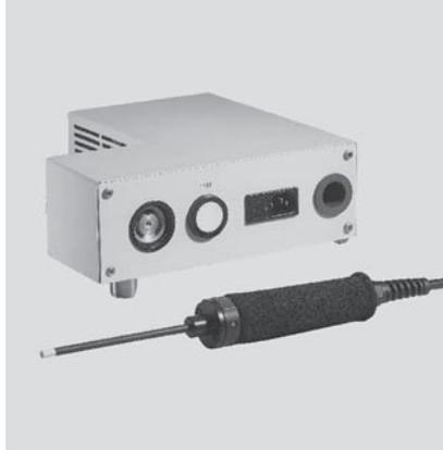
Helium sniffer QUICK-TEST QT 100 with sniffer
