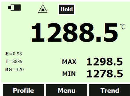
Press <Profile> to enter the first level menu selection. Each displayed name is edited under the PC interface, and then uploads to the instrument. Here the user can continue to the next screen using the arrow keys if the item quantity is more than 15.
