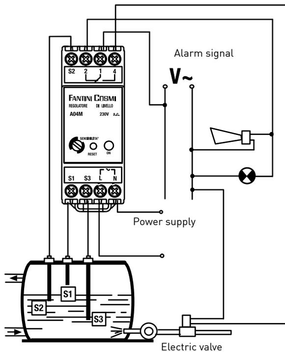
Shutdown level control A04 closes the electric valve and activates an alarm, if the level drops lower than S2.
