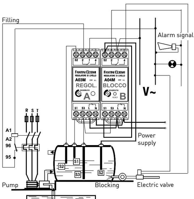
Level control A (A03) regulates the level between S1 and S2; shutdown level control B (A04) interferes to stop the pump and activates an acoustic alarm, if the level drops below the level control's (A04) probe S2.
