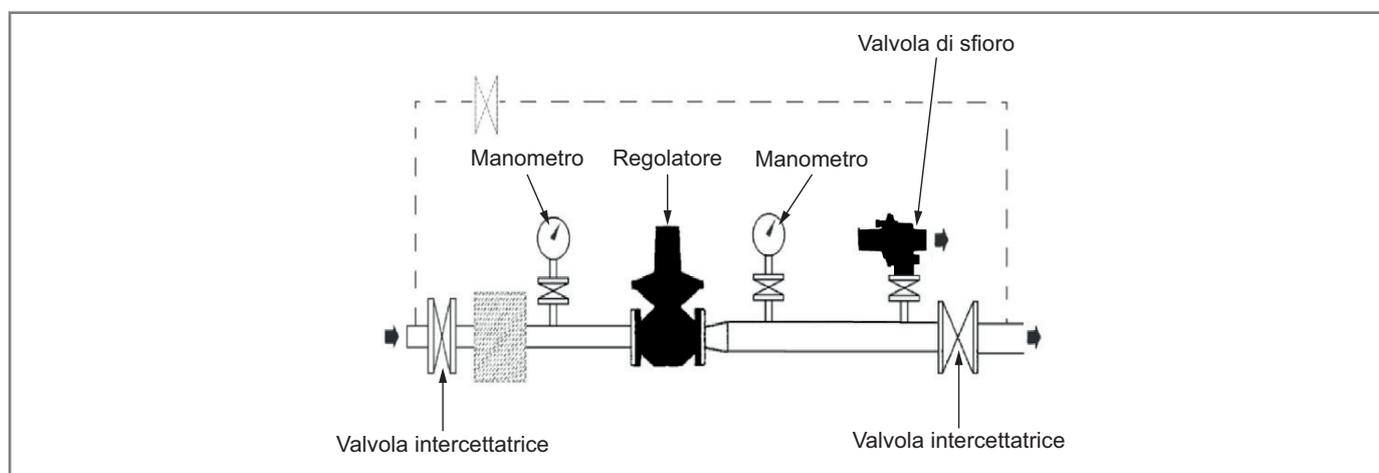
Fig. 6.5. Installation scheme
