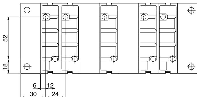
Connection block L and intermediate blocks L and T can be turned so that connection can be made from above or below.
