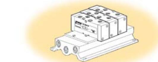
A manifold bar, with common ducts for ports 1, 3 and 5 gives simple, time saving and easily serviced installation. Manifold bars are available in several different sizes, with space for between 2 and 14 valves. They are designed for simple handling and are entirely serviced from the front.
