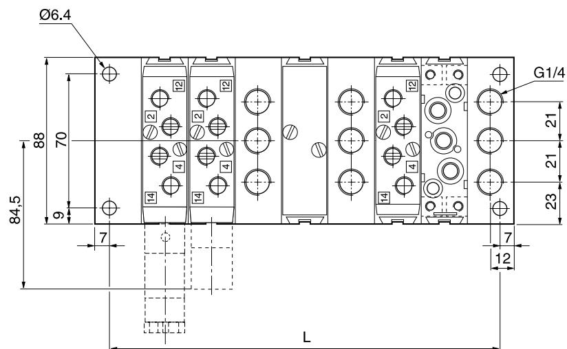
$$L = 34 + (\text{Number of manifolds and Intermediate blocks} \times 24)$$
