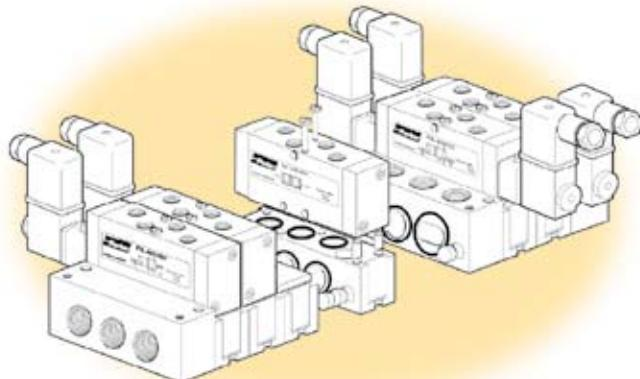
There is a system of multiple installation plates, intermediate blocks and several variants of connectors for the P2L-A. Several variants of connectors are available, which permit connection from above, beneath, straight from the side or in the middle of a valve block. Using the type L manifold, valve blocks may be constructed for supplying several different pressures.
