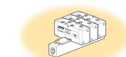
A pressure bar for common primary air supply gives a simple, robust, time saving and easily serviced installation. When pressure bars are used, restrictor-silencers can be installed in the exhaust ports of each valve, for individual adjustment of cylinder/air motor speed. Pressure bars are available in a number of different sizes, with space ranging from 2 to 10 valves.
