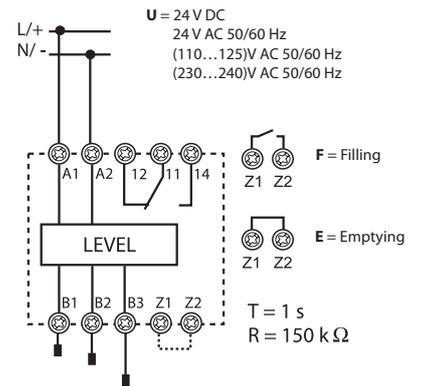
**Special relay for alternating loads, for applications with pumps, compressors, air conditioning or refrigeration units**
