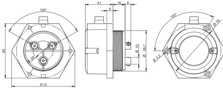
**Electrode and electrode connector**, multiple electrodes may be interconnected to provide required length
