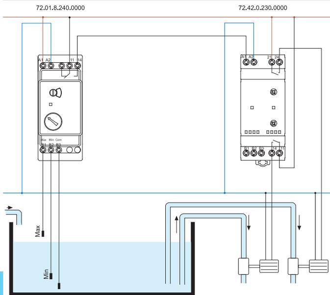
This shows the 72.42 Priority change relay working in conjunction with a single 72.01 level controller. Under normal conditions the liquid level is expected to remain within the range shown as Min to Max. In this case the function of the 72.42 will be to alternate the duty between both pumps, to even wear across both pumps. There is no provision to run both pumps simultaneously.
