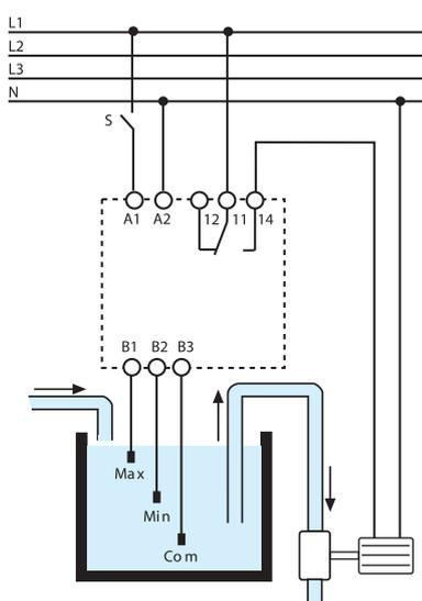
The 72 series level control relays work by measuring the resistance through the liquid, between the common (B3) electrode and Min. and Max. electrodes (B2 and B1). If the tank is metallic, then this can be substituted as the B3 electrode.
