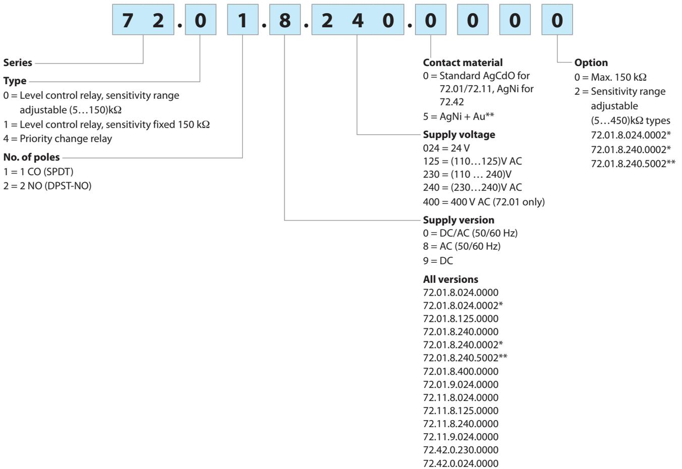
\* For liquids conductivity up to 2 μ Siemens or a Resistance of 450 kΩ
