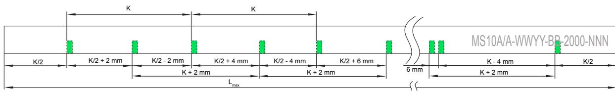
**Multiple reference marks.** For cut reference marks on multiple locations on the MS magnetic scale please contact RLS for a special part numbering.
