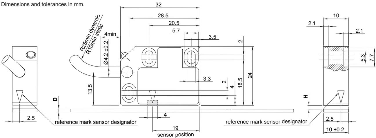
**NOTE:** Ensure recommended M3 readhead fixing screws are tightened to 0.5 Nm to 0.7 Nm.
