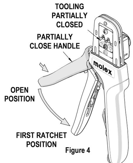
7. Crimp the terminal by squeezing the tool handles until the ratchet mechanism cycle has been completed. Release the handles to open the jaws.
