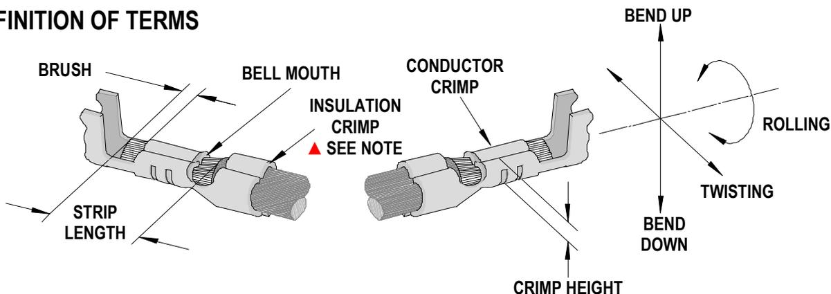
The above terminal drawing is a generic terminal representation. It is not an image of a terminal listed in the scope.
