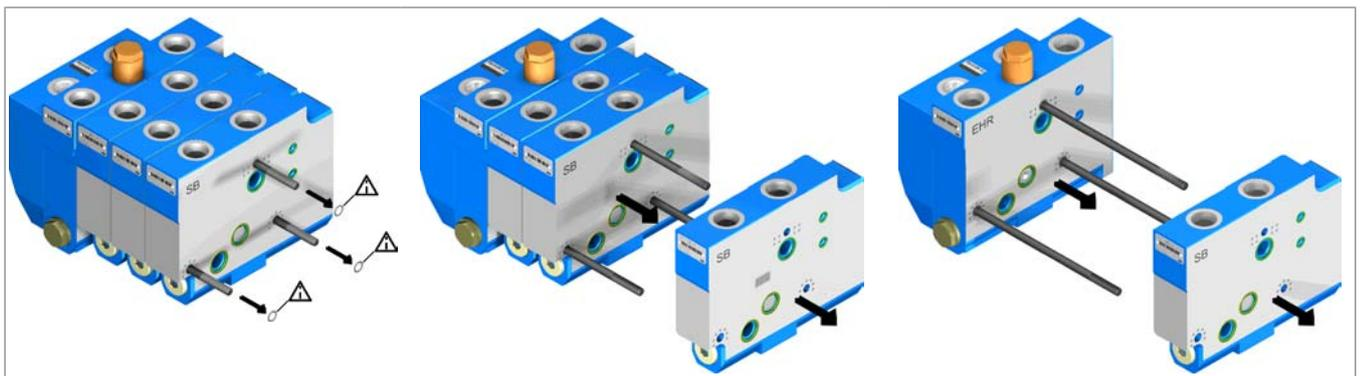
Fig. 2: Control block segment disassembly
