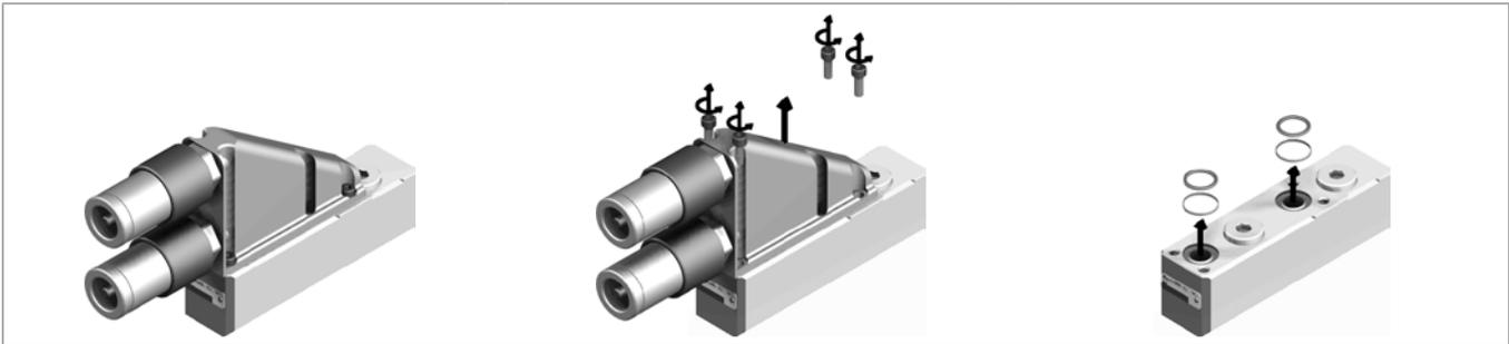
**Fig. 12: Coupling disassembly**
