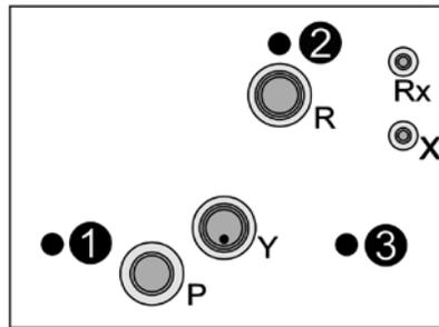
Fig. 8: Flange with three tie rods (Standard)
