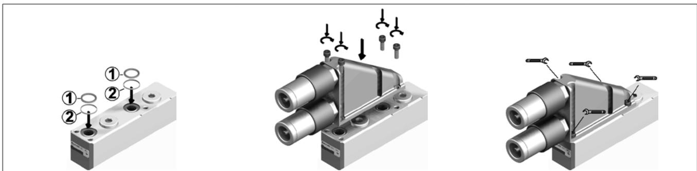
**Fig. 13: Assembly of the customer-specific coupling flange**
