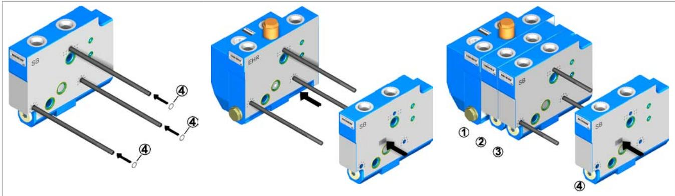
Fig. 6: SB valve assembly
