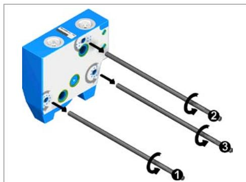
Fig. 3: Subplate disassembly
