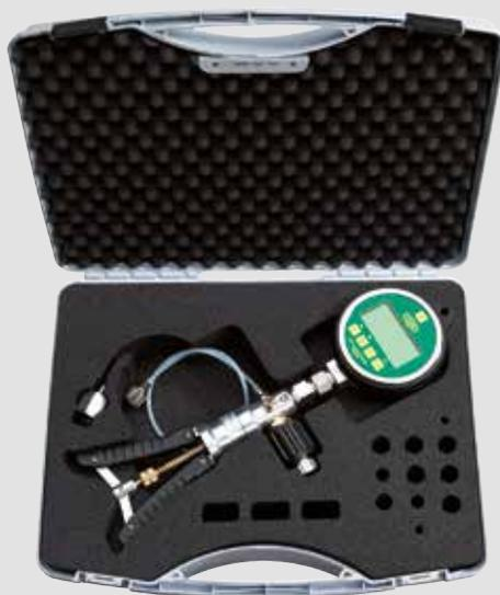
**The REF-CLASS-GAUGE is used to verify the correct calibration of your manifold gauges or any gauges pressure reading. Make sure you are meeting the exact standards of the equipment your servicing!**
