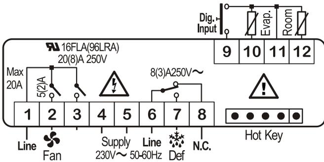
**NOTE:** The compressor relay is 20(8)A or 16(6)A depending on the model.
