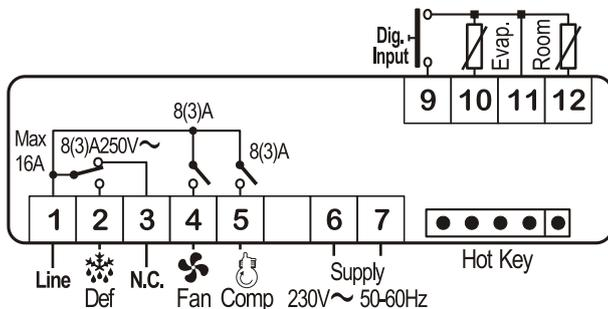
**NOTE:** Connect the 120Vac power supply to 6-7
