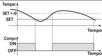
In case of fault in the thermostat probe the start and stop of the compressor are timed through parameters "Cy" and "Cn".
