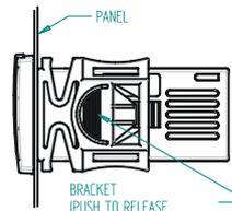
Instrument XR06CX shall be mounted on vertical panel, in a 29x71 mm hole, and fixed using the special bracket supplied. The temperature range allowed for correct operation is 0÷60 °C. Avoid places subject to strong vibrations, corrosive gases, excessive dirt or humidity. The same recommendations apply to probes. Let air circulate by the cooling holes.
